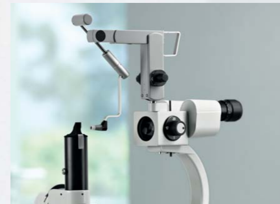
SL 115 Classic with AT 020 applanation tonometer
