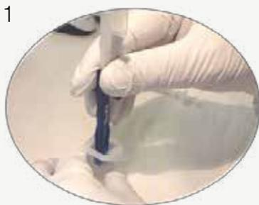
Push the injector vertically in the container as to clip it onto the cartridge.
